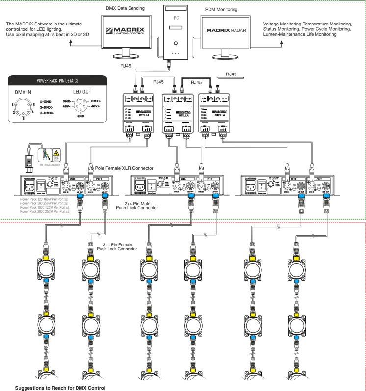
The total cable length should not be more than 3,900 ft (1200m) without buffering.
