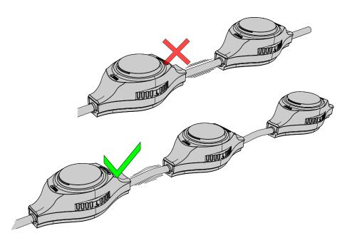
⚠ Do not install by stretching the cables when installing the chain lower module. Install the cables by keeping them as loose as possible.
